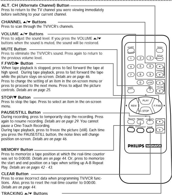
Press during tape playback to adjust the tracking. Details are on page 45.
